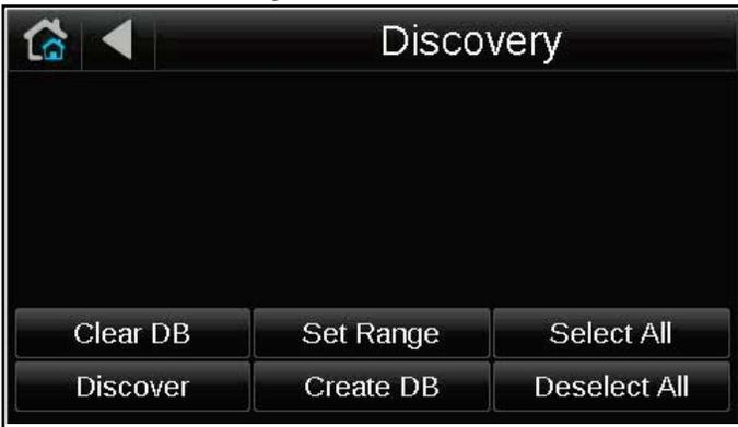
The system will then discover every BACnet controller found on the network. Edit names of discovered controllers if desired by selecting each of the discovered controllers shown on the screen. A key board will appear, rename the device and select **<Done>** when finished. Check the box for all controllers you want on the network or **<Select All>** and click
