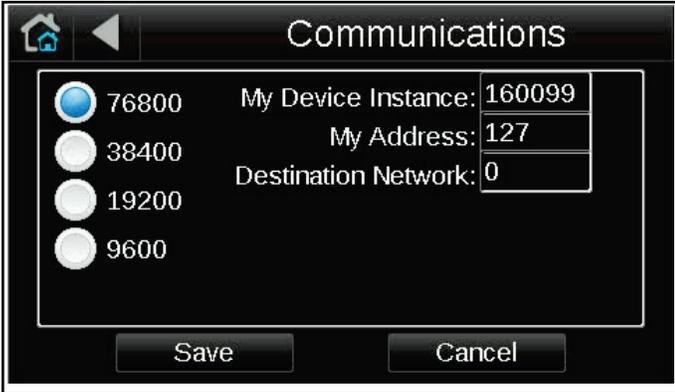
Select the 19200 baud rate and press **<Save>**. This will allow the central panel to communicate with all satellite panels on the network. Check that the baud rate selected matches that set on the control board.
