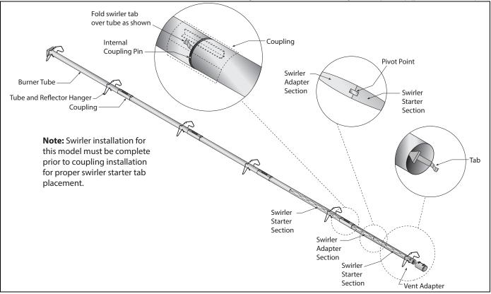
FIGURE 25: Swirler Installation Model: CTH2V-175, 50' Even U-Tube; Swirler Package - 15' (4.5 m) (p/n 03051510K)
