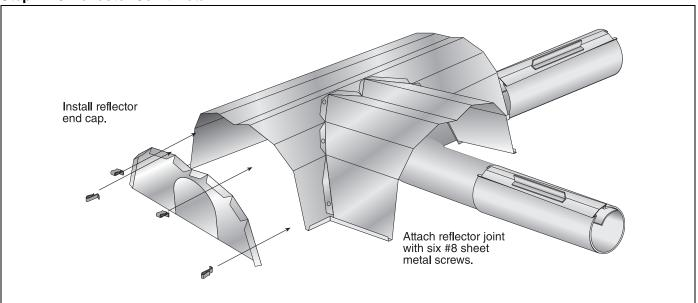
FIGURE 30: Reflector Joint Detail
