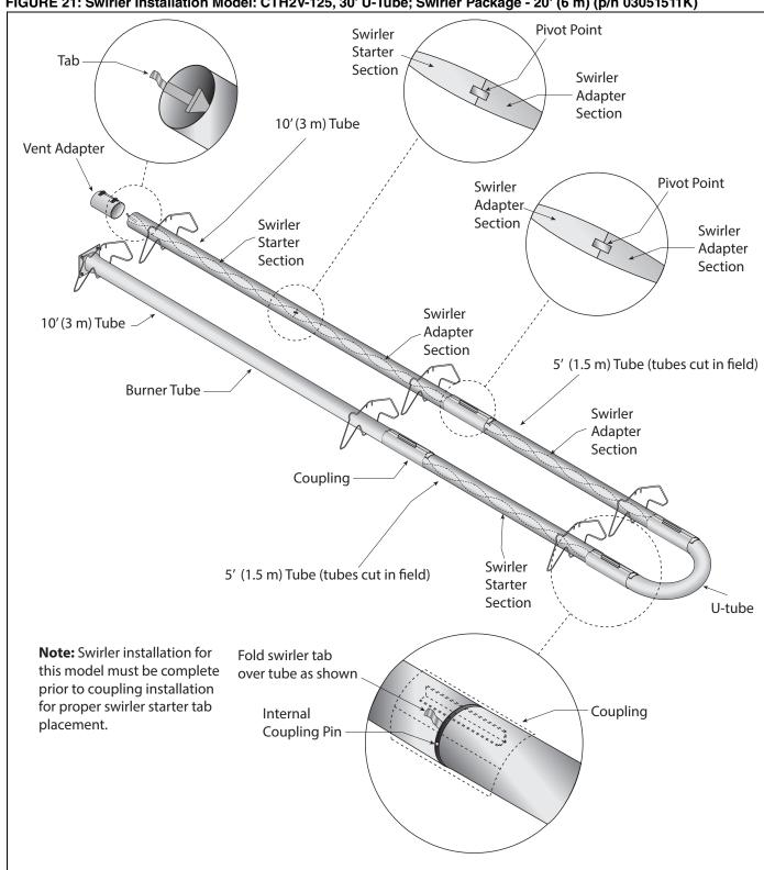
FIGURE 21: Swirler Installation Model: CTH2V-125, 30' U-Tube; Swirler Package - 20' (6 m) (p/n 03051511K)
