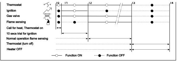
If the flame is not sensed during sequence T2 then the burner will automatically begin re-ignition sequence T1. The ignition sequence will be repeated three times with a 15 second inter-purge. If the flame is not reestablished the heater will go to lockout.
