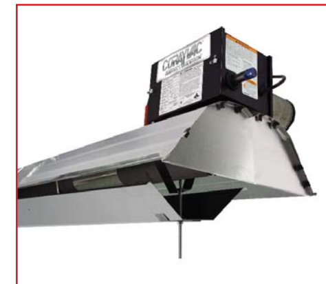
UNIVERSAL SHIELD Universal shields are aluminum reflectors whose angle and height can be adjusted to direct heat to or away from a desired area. Universal shields are available with or without holes.
