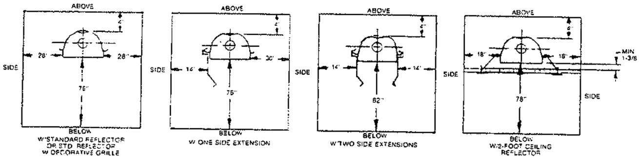
**WARNING:** Minimum clearance from heater must be maintained from vehicles parked below heater.
