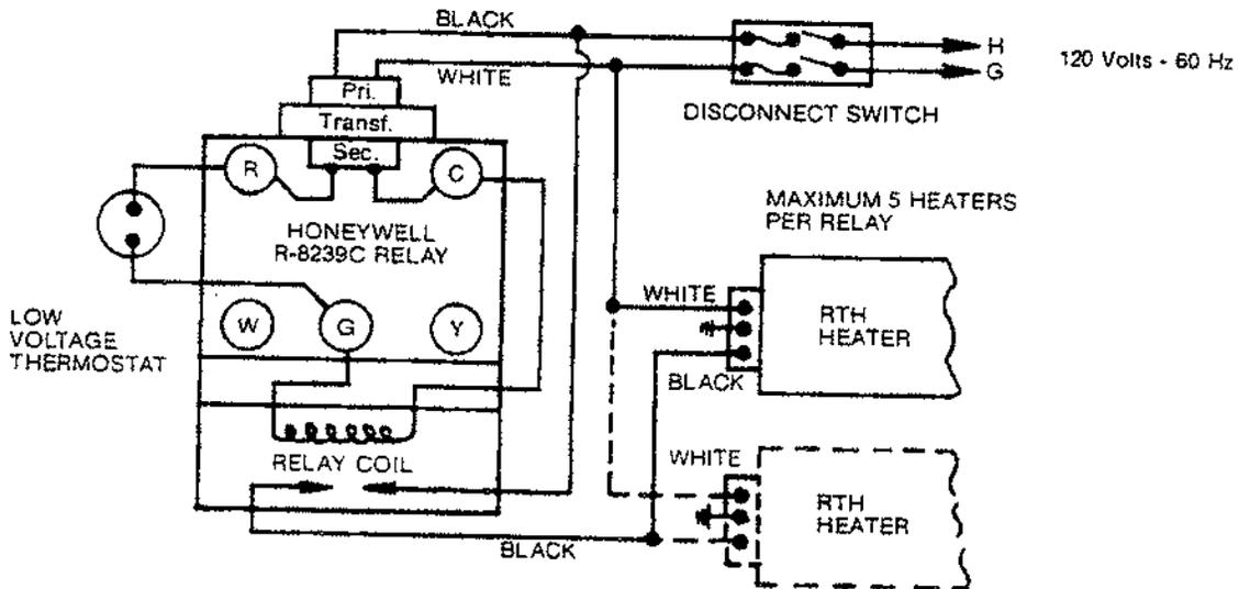
**WIRING OF LOW VOLTAGE THERMOSTAT AND RELAY**
