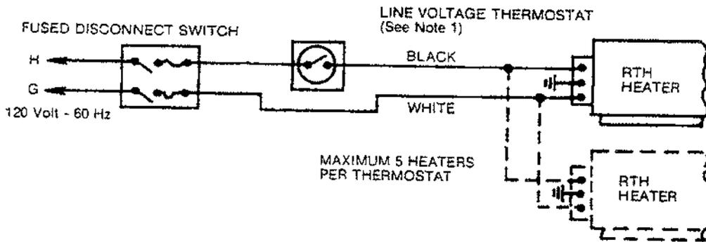
**WIRING OF LINE VOLTAGE THERMOSTAT**
