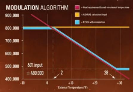
The ROBERTS CORDOL® COMPLETE MODIficating Heating Control also compares outdoor temperature with indoor temperature to operate unitary heaters according to heat load requirements, providing just the right amount of heat for your space conditions.
