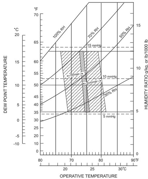
**Fig.4 ASHRAE Comfort Chart Modified for Radiant Heating**
