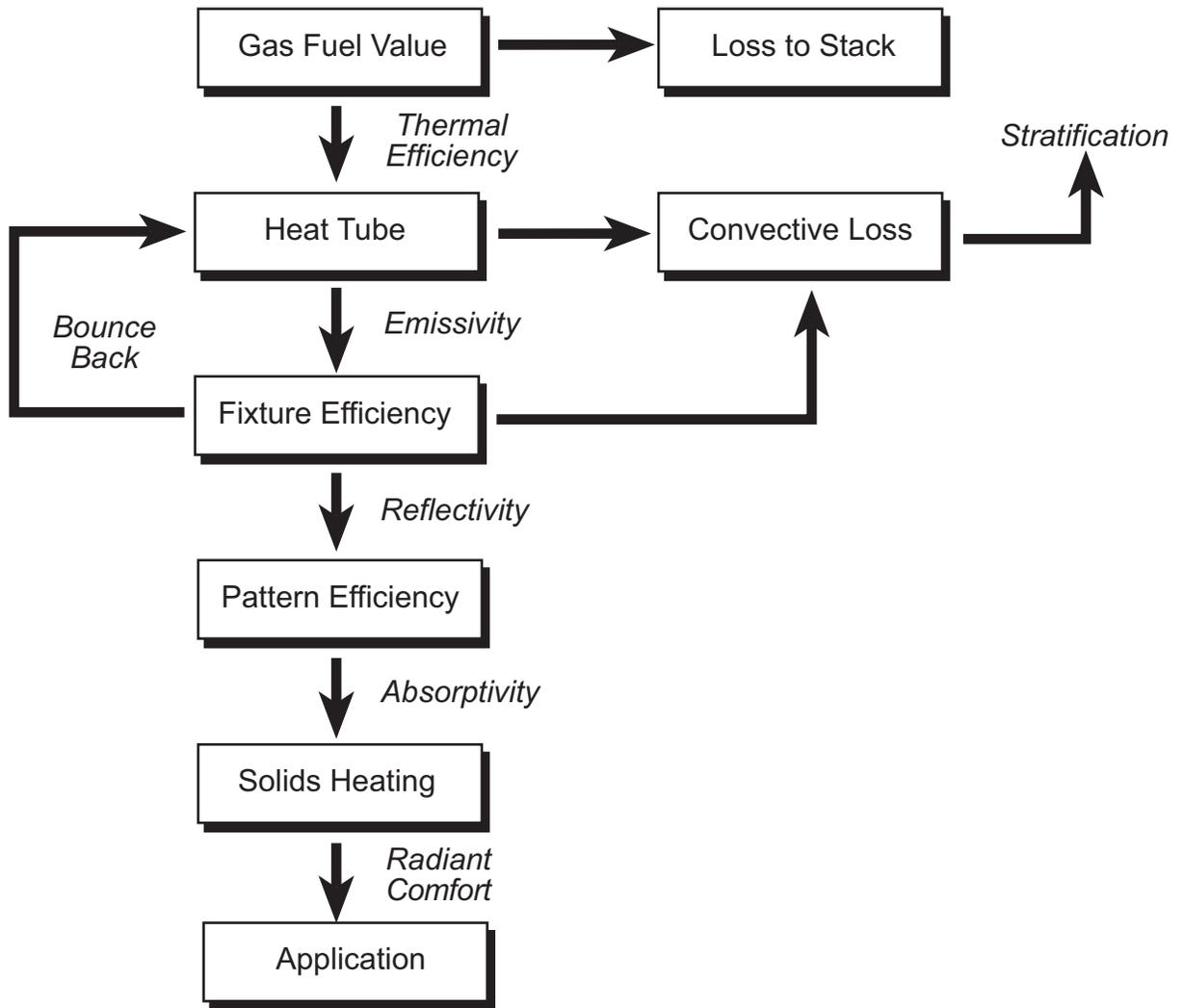
**Figure 2: Energy Flow Chart - Conventional Air Heating**
