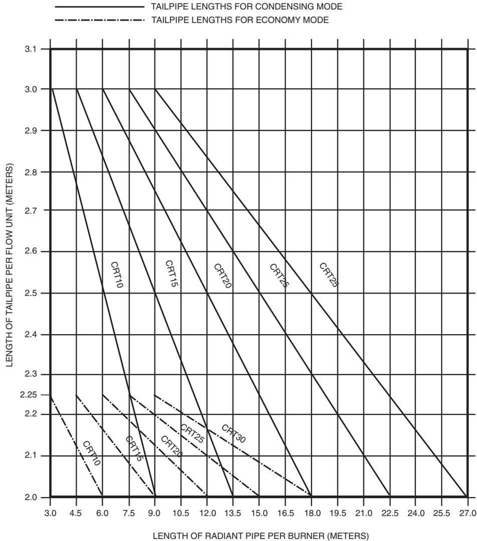
Note: When accounting for the required tailpipe lengths during the design process, it is important to verify that the tailpipe for each branch is at least equal to the specified minimum.
