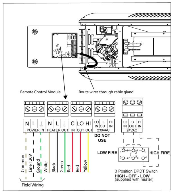
The figure above shows the field wiring connections to the heater remote control module.
