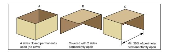
**AWARNING** For the purposes of clearances to combustibles and ventilation all applications not classified as outdoors according to the definitions above shall comply with the requirements for indoor installations.
