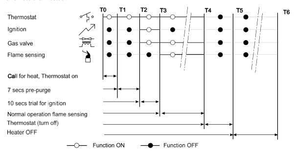
If the burner fails to light, or flame is not detected during the first trial for ignition (a period of 10 seconds) the gas valve is de-energized and the control goes through an inter-purge delay of 15 seconds before another ignition attempt. The control will attempt two additional ignition trials before going into lockout.
