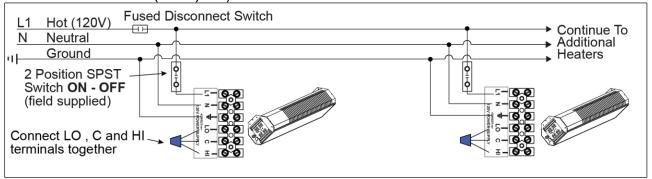
To operate the heater with an individual 120V thermostat use the same connections as above for the switch.
