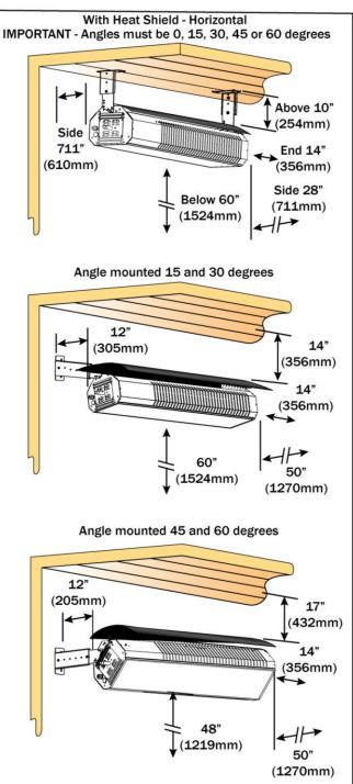
AWARNING The stated clearance to combustibles represents a surface temperature of 117° F (65° C) above room temperature. Building materials with a low heat tolerance (such as plastics, vinyl siding, canvas, tri-ply, etc.) may be subject to degradation at lower temperatures. It is the installer's responsibility to assure that adjacent materials are protected from degradation.
