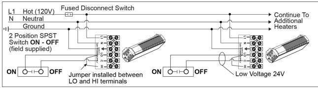
To operate the heater with an individual 24V thermostat use the same connections as above for the switch.
