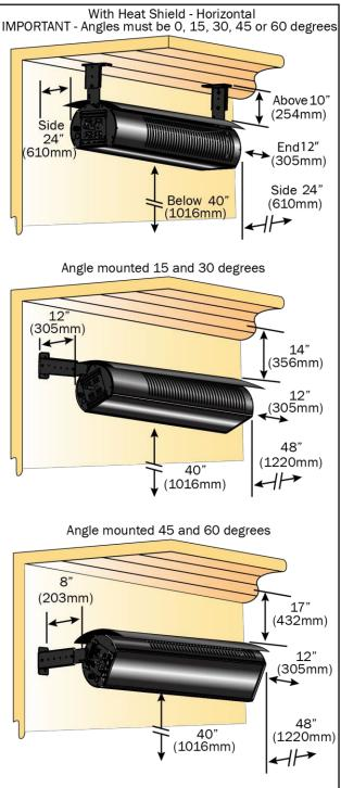
The stated clearance to combustibles represents a surface temperature of 117° F (65° C) above room temperature. Building materials with a low heat tolerance (such as plastics, vinyl siding, canvas, tri-ply, etc.) may be subject to degradation at lower temperatures. It is the installer's responsibility to assure that adjacent materials are protected from degradation.
