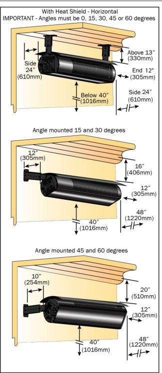
AWARNING The stated clearance to combustibles represents a surface temperature of 90° F (50° C) above room temperature. Building materials with a low heat tolerance (such as plastics, vinyl siding, canvas, tri-ply, etc.) may be subject to degradation at lower temperatures. It is the installer's responsibility to assure that adjacent materials are protected from degradation.
