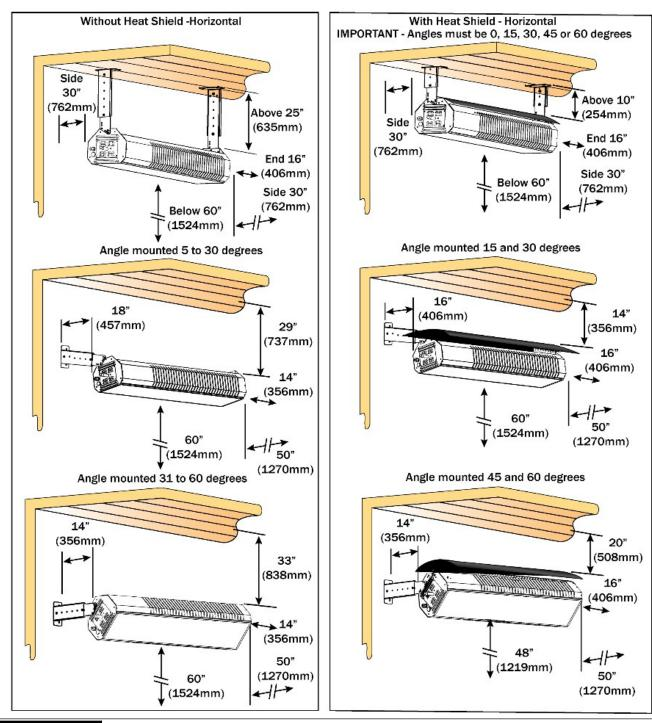
AWARNING The stated clearance to combustibles represents a surface temperature of 90° F (50° C) above room temperature. Building materials with a low heat tolerance (such as plastics, vinyl siding, canvas, tri-ply, etc.) may be subject to degradation at lower temperatures. It is the installer's responsibility to assure that adjacent materials are protected from degradation.
